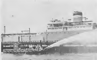
CREW MEMBERS put the new craft through its paces as they approach a dock under full power with turrets throwing salt water under full pressure. The low-built turrets are excellent for fighting fires under the docks. TRIPULANTENAN TA pone e boto nobo na prueba mientras nan ta acerca un dock na fuerza completo cu awa salo ba full presion. E torrennan construi abou ta excelente pa combati candela ba docknan.
